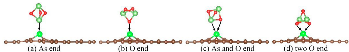
Fig. 4. Four possible adsorption configurations of \text{As}_2\text{O}_3 on Fe/GS.
