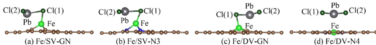
Fig. 8. The most stable adsorption configurations of \text{PbCl}_2 on four types of Fe/GS.
