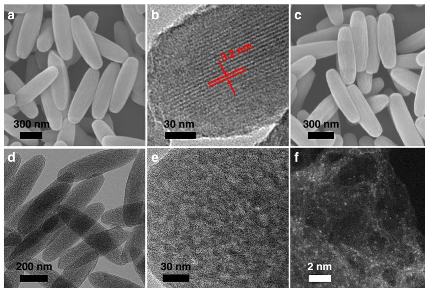
**Fig. 2 Microscopic characterizations.** **a** Scanning electron microscopy (SEM) and **b** transmission electron microscopy (TEM) images of  $\text{PCN-222(Fe)}$ . **c** SEM and **d** TEM images of  $\text{Fe}_{\text{SA}}\text{-N-C}$ . **e** Enlarged TEM image showing the mesoporous structure of  $\text{Fe}_{\text{SA}}\text{-N-C}$ . **f** Aberration-corrected HAADF-STEM image of  $\text{Fe}_{\text{SA}}\text{-N-C}$ .
